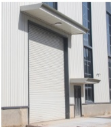
Electric rolling shutter door
