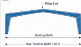
1 Tapered Column Clear Span (TCCS)
