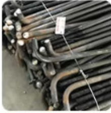
Embedded bolts for foundation
