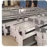
Structure frame for columns or beams
