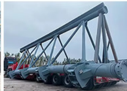
9. Spray paint and galvanize steel structure according to technical requirements of drawings
