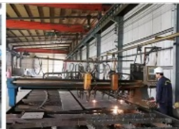
3. According to the drawing specification, laser cutting into the corresponding component size
