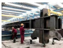
8. Inspect welded steel structure, prepare for galvanizing or painting
