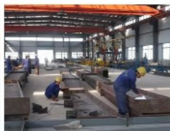
5. The steel plate was shot blasted to remove rust
