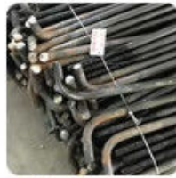
Embedded bolts for foundation
