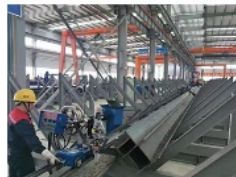
4.Drill holes into some steel plate parts
