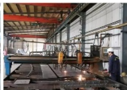
3. According to the drawing specification, laser cutting into the corresponding component size
