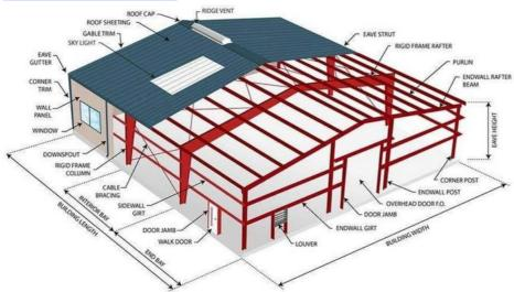
This Steel Structure warehouse comes with a surface treatment of either Hot Dip Galvanised or Painted, which makes it resistant to rust and corrosion. The steel is treated through a process that involves dipping it in molten zinc, which forms a protective layer on the surface, preventing it from rusting and corroding. The paint coating also provides additional protection against the elements and helps to enhance the aesthetic appeal of the building.
